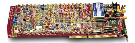
*Model* 4481-*P70/Q* is a tunable IF telemetry receiver module for the ISA bus. When combined with SBS Technologies Model 4422-PCI Telemetry Module, all of the functions of a satellite ground station are provided in just two PC bus slots.
